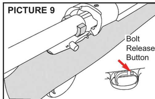
6. Push the bolt assembly forward until the bolt stop is engaged, and the bolt assembly is locked into the receiver.
