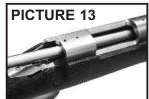
**WARNING!** The breech plug must be seated correctly in the barrel to ensure the proper and safe operation of the firearm. Do NOT attempt to discharge the rifle if the breech plug will not thread in smoothly and or tighten snugly to 100 in-lbs. If the breech plug cannot be seated or secured correctly, see “Repair Services” on page 32. Discharging a firearm with a breech plug not secured correctly may lead to property damage, personal injury, and/or death.
