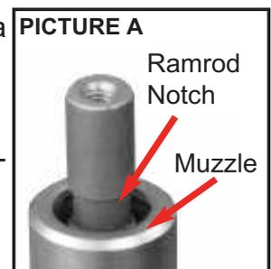
If the single wide notch near the end of the ramrod is even with the muzzle, then the firearm is unloaded and does not have an obstruction.
