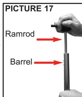
**Note:** Reference marks are provided on the ramrod for a full load depth. Use these markings as a reference after each loading.
