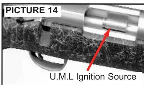
17. Close the bolt by pushing it fully forward then rotate the bolt handle down, locking the bolt into position and the ignition source onto the nipple.
