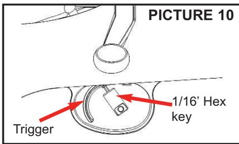
8. Adjust the trigger pull force to the desired setting by turning the adjustment screw:
