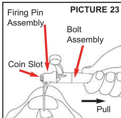
3. While pulling the bolt body, the firing pin head will be pulled away from the bolt body, place a coin into the slot in the right side of the firing pin assembly. See Picture 23.
